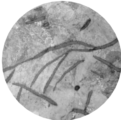
Photomicrograph showing graphite form in gray iron.
