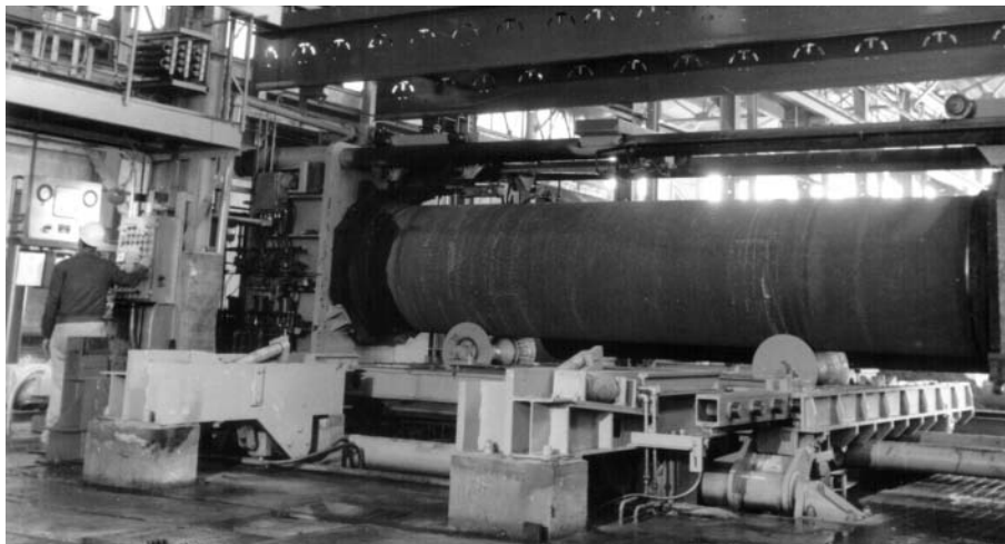
Each 30" and larger diameter AMERICAN Ductile Iron pipe is hydrostatically tested to 75% of yield strength which results in higher test pressures than those required by AWWA C151, varying to over 900 psi, depending on size and thickness of the pipe.
